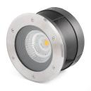
LED recessed lamp with a beam angle of 24° for garden and terrace lighting, built in 316 stainless steel and glass. The light source is 24W COB LED and warm light. Flush mount box and driver are included. This LED floor - recessed lamp is ideal for creating guide lights which highlight the paths in gardens and building areas. This luminaire features IP67 that gives high protection against rain and solids. It comes with IK08 shock resistance. Permits vehicle passage up to 1000Kg.
