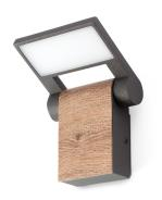
WOOD is a trendy LED wall lamp for outdoor lighting, made of aluminium with a polycarbonate diffuser. The light source is SMD LED 10W 3000K 600Lm CRI>80. This wall lamp projects a beam of light through the bottom areas to provide both decorative and functional lighting. Can be directed once installed and has the box accesory.
