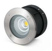
LED recessed lamp with a beam angle of 60° for garden and terrace lighting, built in 316 stainless steel and glass. The light source is 12W COB LED and warm light. Flush mount box and driver are included. This LED floor - recessed lamp is ideal for creating guide lights which highlight the paths in gardens and building areas. This luminaire features IP67 that gives high protection against rain and solids. It comes with IK08 shock resistance. Permits vehicle passage up to 1000Kg.
