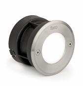
LED recessed lamp for garden and terrace lighting, built in 316 stainless steel and glass. The light source is HIGH POWER LED 3W and cold light. Flush mount box and driver are included. This LED floor - recessed lamp is ideal for creating guide lights which highlight the paths in gardens and building areas. This luminaire features IP67 that gives high protection against rain and solids. It comes with IK08 shock resistance. Permits vehicle passage up to 1000Kg.
