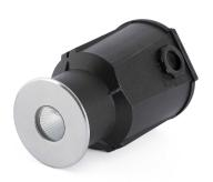
LED recessed lamp for garden and terrace lighting, built in 316 stainless steel and glass. The light source is COB LED 7W 3000K 280Lm CRI >80. Flush mount box and driver are included. This LED floor - recessed lamp is ideal for creating guide lights which highlight the paths in gardens and building areas. It comes with IK08 shock resistance. Permits vehicle passage up to 600Kg.
