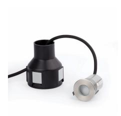
LED recessed lamp for outdoor lighting with LED technology and warm light, made of cast aluminium and 316 stainless steel, with tempered glass diffuser. ABS flush mount box included. The light source is LED 3000K 2W 65Lm 120°. It comes with IK08 shock resistance. Permits vehicle passage up to 1400Kg.
