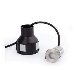
Modern recessed lamp with LED technology and warm light, for outdoor lighting, made of 316 stainless steel and aluminum, with tempered glass diffuser. ABS flush mount box included. The light source is HIGH POWER LED 2W 3000K 77Lm. It comes with IK08 shock resistance. Permits vehicle passage up to 1400Kg.
