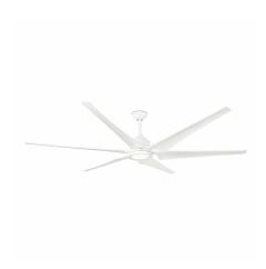
Ceiling fan with light and DC motor suitable for rooms from 28m2. The colour of blades are white, not reversible. Operated by remote control (included) setted up with 5 dimmable speeds 6 - 9 - 15 - 28 - 44W and 54 - 67 - 79 - 98 - 112rpm. This ceiling fan is suitable for inclining roof.
