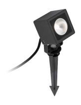
LED Projector with spike and warm light for outdoor lighting made of die cast aluminum with trasparent glass diffuser. The light source is COB LED 7W 3000K 550Lm 50° CRI>80. This adjustable projector is ideal for garden lighting and it allows you to enhance decorative elements. This luminaire features IP65 that gives high protection against rain and solids.
