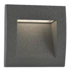
Wall recessed lamp with LED technology for garden and terrace lighting, built in aluminium. The light source is SMD LED 3W 3000K 122Lm. Flush mount box and driver are included. This LED recessed lamp is ideal for outdoor signal lighting. This luminaire features IP65 that gives high protection against rain and solids.
