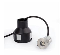
CURTIS is a LED recessed lamp asymmetric with warm light, for outdoor lighting, made of 316 stainless steel and aluminum, with tempered glass diffuser. ABS flush mount box included. The light source is HIGH POWER LED 2W 3000K 77Lm. It comes with IK08 shock resistance. Permits vehicle passage up to 1400Kg. This exterior recessed lamp is ideal to obtain a wall - washing effect.
